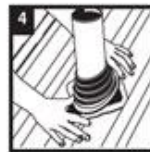
4 Form flashing to roof profile
