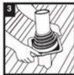
3 Slide flashing over Pipe using water.
