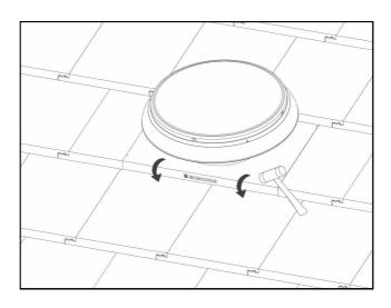
To ensure a weatherproof installation, apply a bead of silicone under the side and front edges of the flashing.
