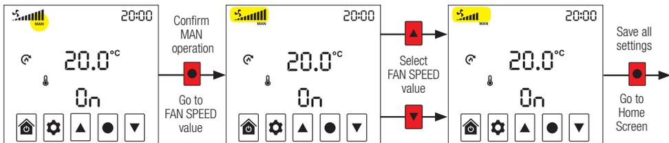
Fan speed will remain constant at the speed set. If system is in BOOST mode, the fan will operate at the speed set for that mode.
